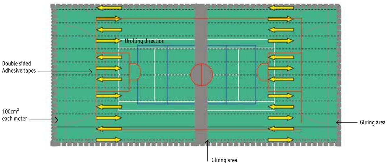
We recommend a dual-component epoxy glue, GreenLay Glue, reference Component A 1551057 Component B 1551058 – quantity to be applied, with a thin set of teeth spatula, between 300 and 350 gr per sqm. For a good installation you must carefully follow the manufacturer recommendations in particular, the waiting time before applying the covering. Then compact the surface with a roller to eliminate any bubbles that might remain between the sub-floor and the covering.
